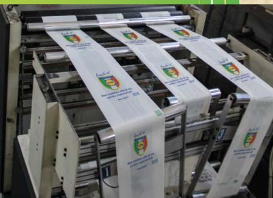
MACCHINA IN LINEA DA STAMPA E SALDATURA
