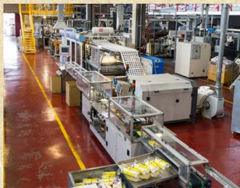
ESTRUSORE E TERMOFORMATRICE IN LINEA PER BICCHIERI IN BICOMPOST
